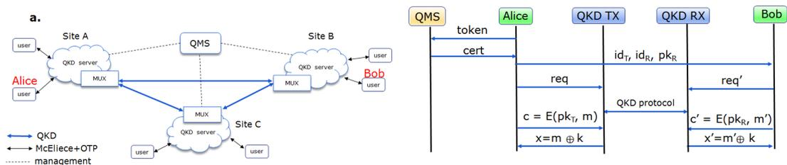
**Fig. 1.** a. A system model for QKD as a service. QMS stands for QKD Management Server. b. A key agreement protocol.
