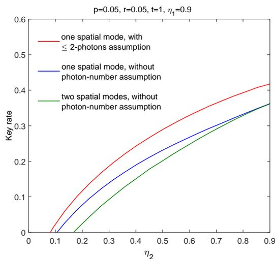
FIG. 2: Key rate as a function of the detection efficiency  $\eta_2$  of the second detector (for the optical signals in the first spatial mode) in the active-detection scheme. Here we fix the efficiency of the first detector (for the optical signals in the first spatial mode) to  $\eta_1 = 0.9$ . See the text for other details.
