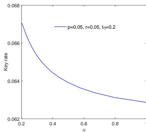
FIG. 1: Key rate as a function of the detection efficiency  $\eta$  of each detector. Here we keep the product of detection efficiency  $\eta$  and transmission efficiency  $t$  fixed, so the observed distribution is the same for all values of  $\eta$  plotted.
