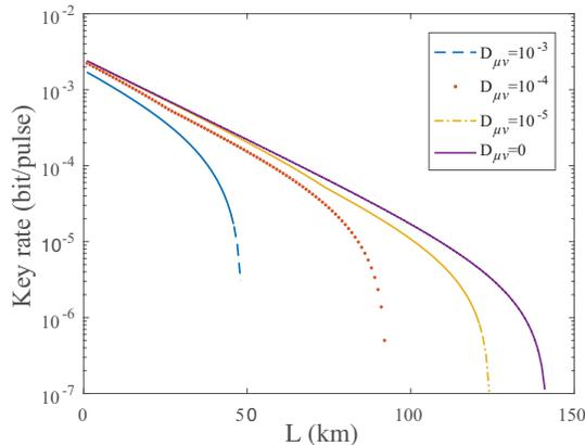
FIG. 3. Estimated key rate for different  $D_{\mu\nu}$ . The parameters used here are the same as in Fig. 2. The intensities of the signal state and the decoy state are optimized with step 0.01 from  $\mu \in [0.01, 0.5]$ ,  $\nu \in [0.01, 0.2]$ .
