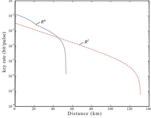
FIG. 2. Lower bound  $R^l$  and optimized upper bound  $R^u$  of key rate. The parameters used in the simulation are from the GYS experiment [12], which are  $Y_0 = 1.7 \times 10^{-6}$ ,  $e_0 = 0.5$ ,  $\eta_{Bob} = 0.045$ ,  $e_{detector} = 0.033$  and  $f(E_\mu) = 1.22$ . The quantum channel loss is 0.21 dB/km. The mean photon numbers are  $\mu = 0.6$  for the signal state and  $\nu = 0.2$  for the weak decoy state.
