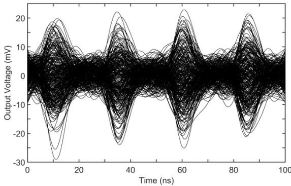
Fig. 1 Time traces of the homodyne detector output at a repetition rate of 40 MHz (The LO power is  $8 \times 10^7$  photons per pulse).
