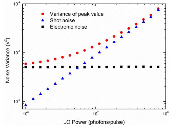
Fig. 2 The output peak value variance of the detector versus the LO power for vacuum field input.
