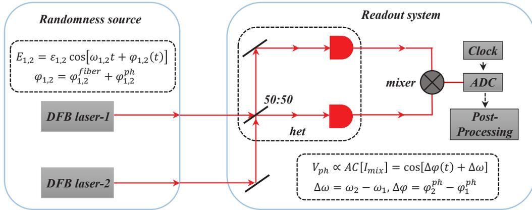
Fig. 1. The experimental setup of phase noise based QRNG without delay line, where the mixer is used to generate the final random voltage. The 12-bit analog-to-digital converter (ADC) is also used with the sampling rate of 100MHz
