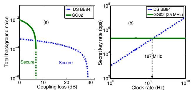
Fig. 3. (a) Regions of secure operation for decoy-state BB84 and GG02 protocols in setup 2. The curves show the maximum tolerable background noise at different values of coupling loss. (b) Comparison of the two systems when the CV repetition rate is fixed to 25 MHz at 5 dB coupling loss.
