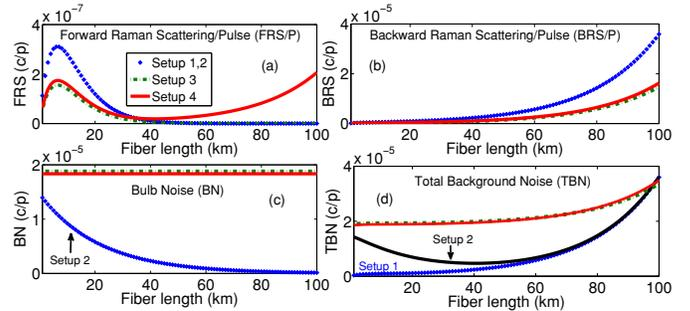
Fig. 2. Noise counts due to (a) forward Raman scattering, (b) backward Raman scattering, (c) the artificial lighting source at  $10^{-5}$  W/nm of power spectral density, and (d) the total background noise at 10 dB coupling loss.
