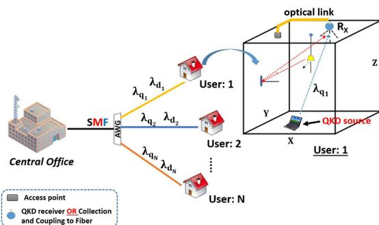
Fig. 1. Schematic view of exchanging secret keys between an indoor wireless user with a central office at the end of an access network.
