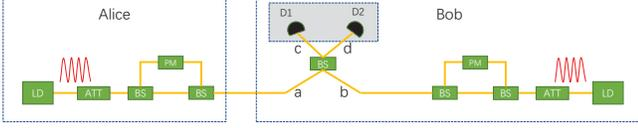
Figure 1. Passive RRDQPS-QKD scheme. Alice and Bob use a local laser to generate an L-pulse reference independently, which are then encoded to time-bin of X or Y basis by AMZI. Bob records the coincidence clicks. LD: laser diode; ATT: variable attenuator; BS: a 50/50 beam splitter (fiber); PM: phase modulator; D1 & D2 in gray box means these two detector are untrusted.
