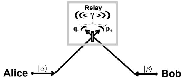
FIG. 1: In a prepare-and-measure CV MDI QKD protocol, Alice and Bob send coherent states  $|\alpha\rangle, |\beta\rangle$  (corresponding to the variables  $X$  and  $Y$  respectively) to the relay. The relay applies a Bell measurement to the incoming signals, and broadcast the result  $\gamma$  (corresponding to the variable  $Z$ ) to Alice and Bob.
