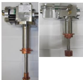
Figure 1. Photos of a compact and an existing RDK-101 GM expander.
